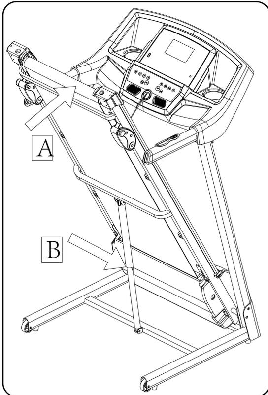
Pull up the base frame at position A, till hearing the sound that the air pressure bar B is locked into the round tube
