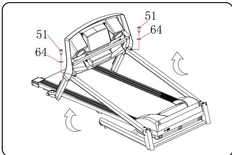
1、 Holding the computer frame and uprights, unscrew bolt M8\*16(51) and lock washer (64) off right uprights, use the 5# Allen wrench to lock the computer and upright tube tight by screw M8\*16(51) and lock washer (64) See as left picture.
