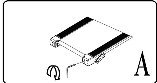
If the belt has drifted to the left, turn the left adjusting bolt 1/4 turn clockwise, then start running until centering the belt. Pic B
