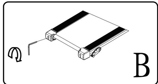
Timely adjust the tightness of the belt, if need, turn the left and right adjusting bolt 1/4 turn clockwise, then re-start running, confirm the belt-tightness until the belt be right tightness. Pic C
