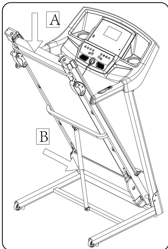
Support place A with hand , kick the place of air pressure bar, then the main frame will fall down automatically ( Please keep anybody and any pet away the machine when falling down)
